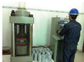
芯样和试块强度检测 Core and Cube Strength Testing
